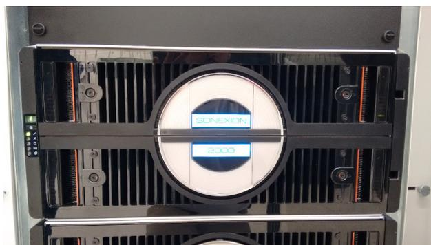
Figure 1. Cray Sonexion 2000 Scalable Storage Unit (SSU).
