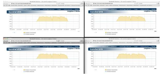
Figure 15: Write Bandwidth for all four Longbow links when running two GPFS clients.
