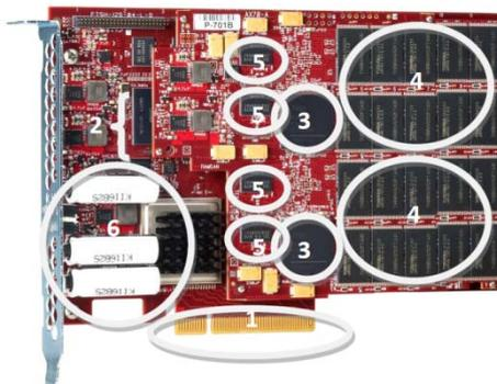
**Figure 3:** RamSan-70 card. 1=PCIe 2.0 x8, 2=PowerPC CPU, 3= FPGA, 4=450 usable Flash (650 raw), 5=RAM, 6=Super capacitors
