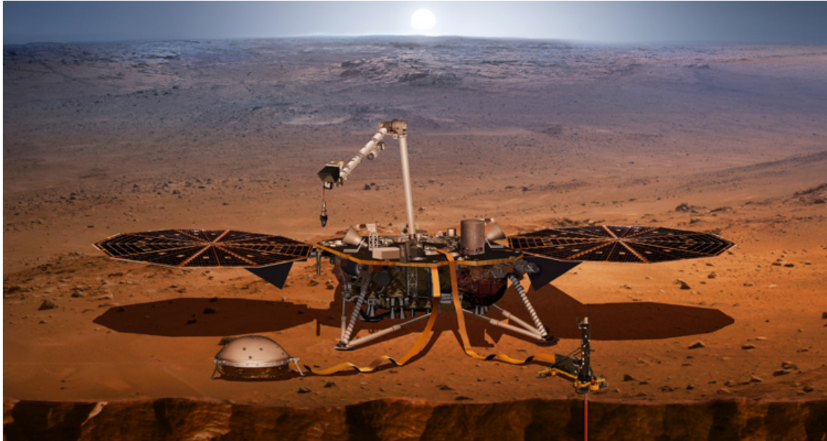
Artist's rendering of the InSight lander. The sensor assembly of the seismometer (underneath the protective shield) is pictured at the front left. (Image: NASA/JPL-CALTECH)
