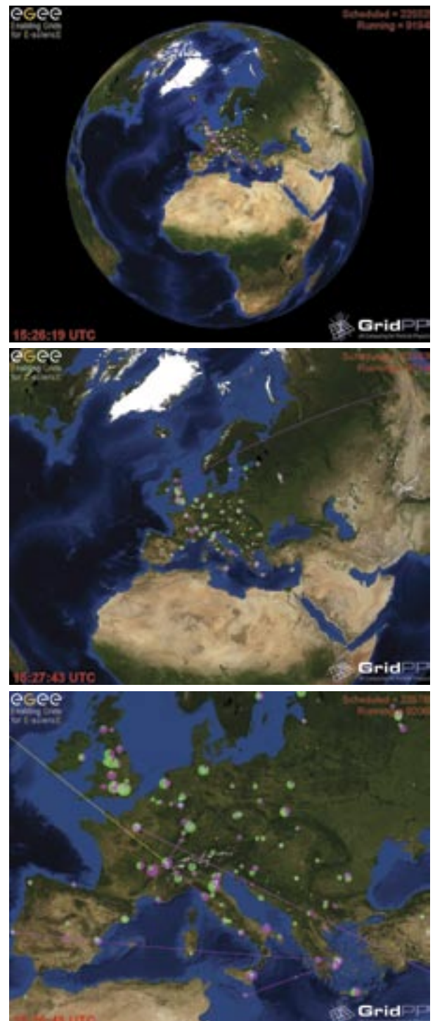
The EGEE real-time monitor represents each institution running a Grid 'node' as a pulsating colored dot, which alternates between green and red, depending on the load of the system. The lines connecting nodes represent active data transfer operations.
