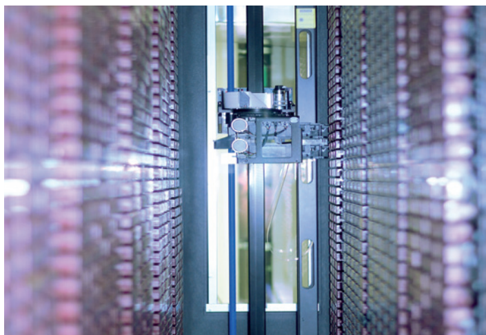
The new IBM Tape library TS3500 with its 5000 tapes.
