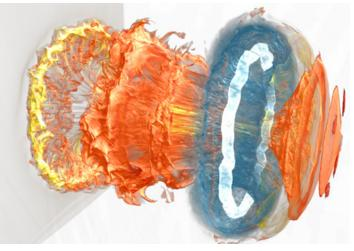
What might look like an especially flamboyant jellyfish is actually a scientific simulation of flow phenomena. This extraordinarily detailed computer simulation conducted on supercomputers of CSCS, demonstrates what happens when a air shock wave hits a helium bubble. Similar phenomena are involved in rapid combustion processes or shattering kidney stones with shockwave lithotripsy, for instance. (*Image: Diego Rossinelli, Computational Science and Engineering Laboratory, ETH Zurich*)
