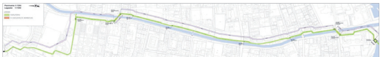
The water pipe (green) stretches 2.8 km across the city to connect the lake (right) with the computing centre. On its way it crosses under the Cassarate river twice.
