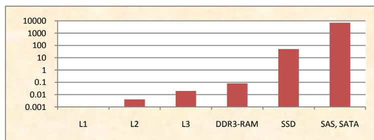
Figure 1: Typical latency in  $\mu$ s for several storage devices
