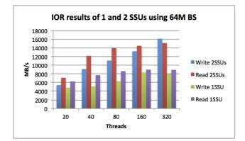
Figure 6. IOR read and write performance on one and two SSUs with 64MB block size and up to 320 client-side hardware threads distributed across the 20 client nodes.
