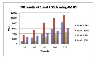
Figure 4. IOR read and write performance on one and two SSUs with 4MB block size and up to 320 client-side hardware threads distributed across the 20 client nodes.
