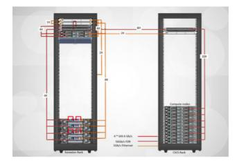
Figure 2. Schematic showing Sonexion 2000 test bed rack layout and connections to CSCS' x86 test cluster.
