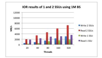
Figure 3. IOR read and write performance on one and two SSUs with 1MB block size and up to 320 client-side hardware threads distributed across the 20 client nodes.
