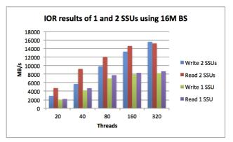
Figure 5. IOR read and write performance on one and two SSUs with 16MB block size and up to 320 client-side hardware threads distributed across the 20 client nodes.
