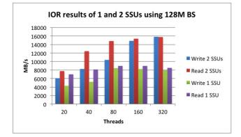
Figure 7. IOR read and write performance on one and two SSUs with 128MB block size and up to 320 client-side hardware threads distributed across the 20 client nodes.
