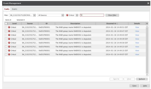
Figure 13. Simulating the failure of 8 disks in 8 RAID arrays.
