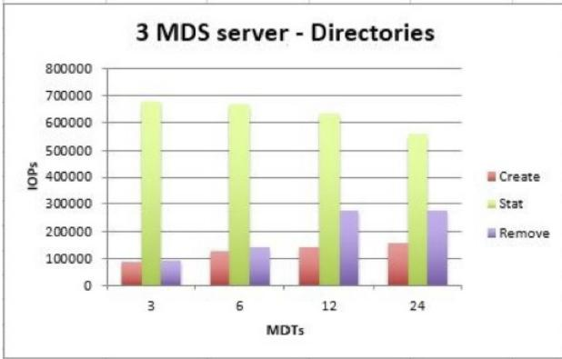
Figure 11. mdtest results for directory operations using a 3 metadata servers (MDSs) having from 3 to 24 metadata targets (MDTs), i.e. 1 to 6 director blades.
