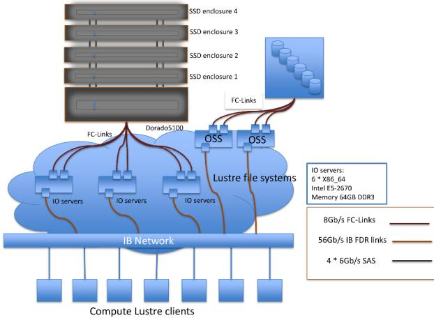
Figure 5. Schematic showing the test environment used for the Lustre testing including IO servers, Dorado5100 as metadata storage, some additional data storage and compute clients.
