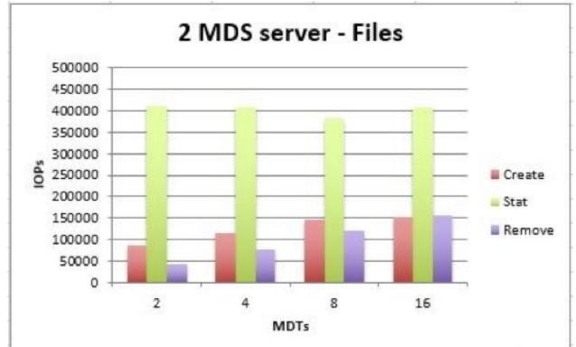
Figure 10. mdtest results for files operations using a 2 metadata servers (MDSs) having from 2 to 16 metadata targets (MDTs).
