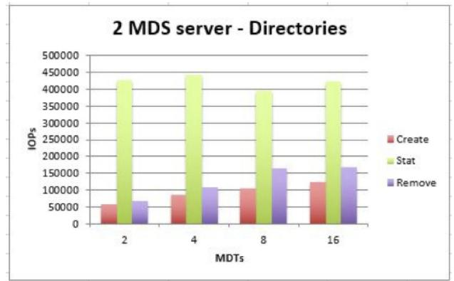
Figure 9. mdtest results for directory operations using a 2 metadata servers (MDSs) having from 2 to 16 metadata targets (MDTs).
