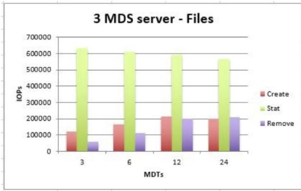
Figure 12. mdtest results for file operations using a 3 metadata servers (MDSs) having from 3 to 24 metadata targets (MDTs), i.e. 1 to 6 director blades.
